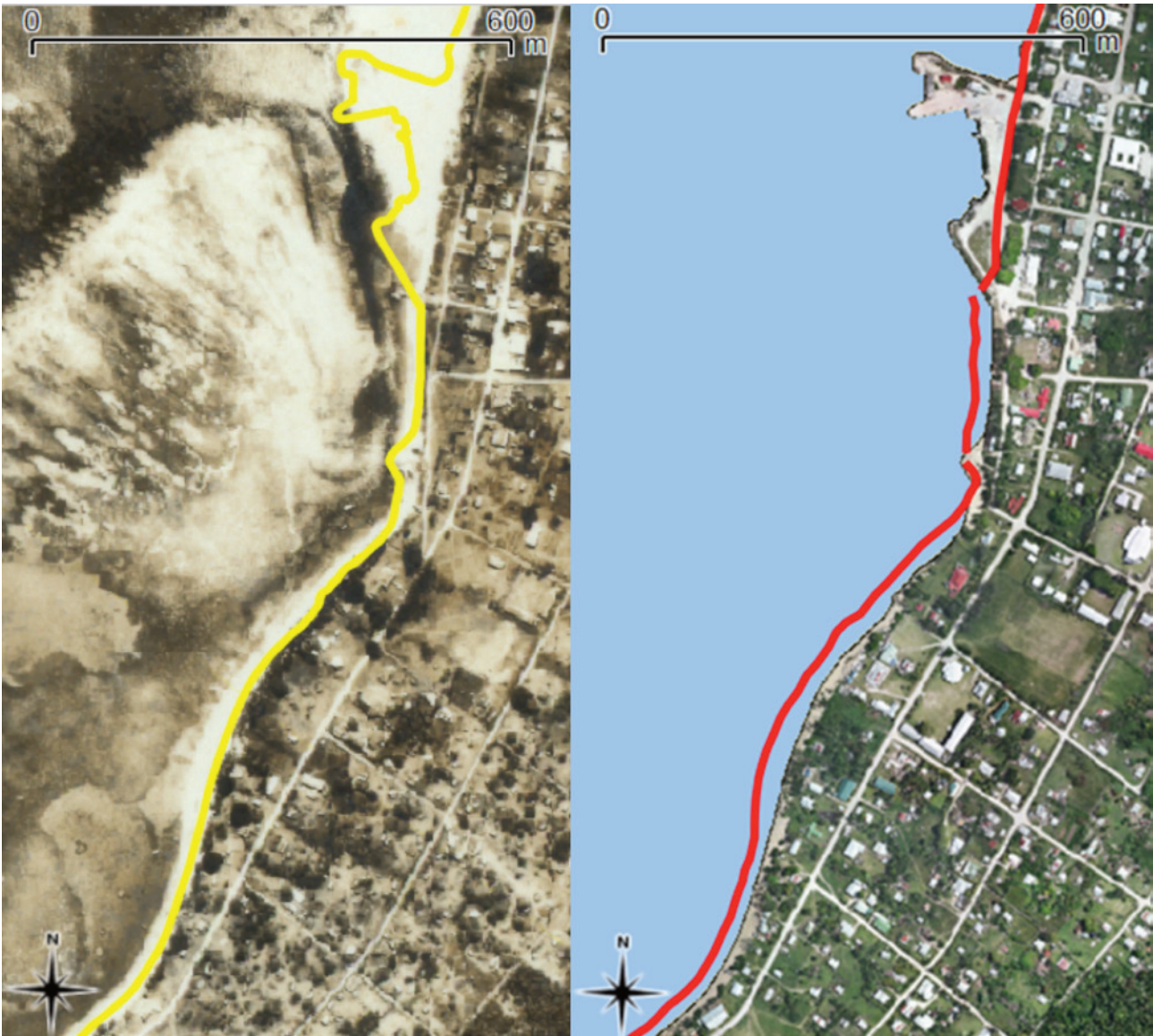
Figure 19: On the left, Pangai in 1968 with the 2011 shoreline superimposed. On the right, Pangai in 2011 with the 1968 shoreline superimposed. Note that the old piled jetty visible in the top third of the 1968 image was replaced by a stone causeway in 1982, and that the present Pangai Harbour, opened in 1996, is visible near the top of the 2011 image.
