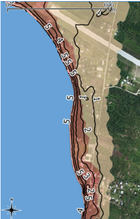
Figure 32: Koulo and Holopeka flood depths in metres, 2100, based on an intermediate–high sea-level rise scenario and severe tropical cyclone conditions (see text for details)
